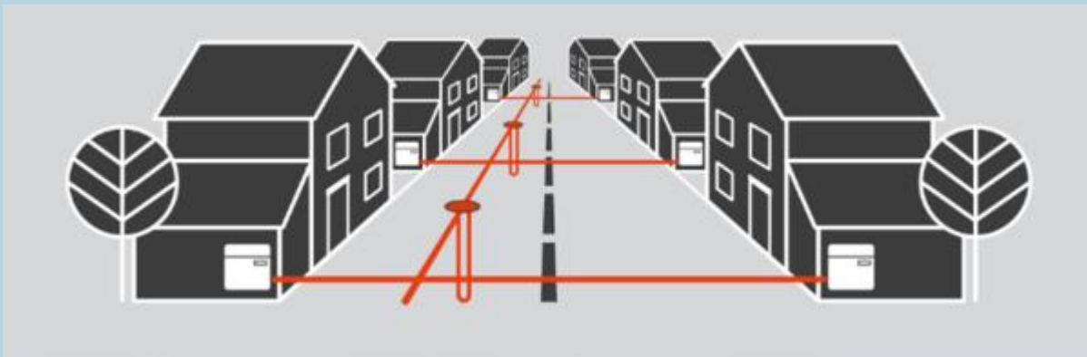
Figure 6-10 Ground Source Heat Pumps + Shared Ground Array
