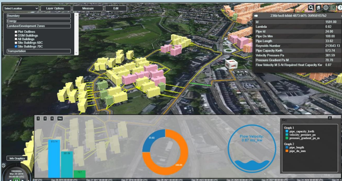
Figure 7-21 Example dashboard for the digital twin for Caerau (Bridgend) – providing information regarding a district heat network
