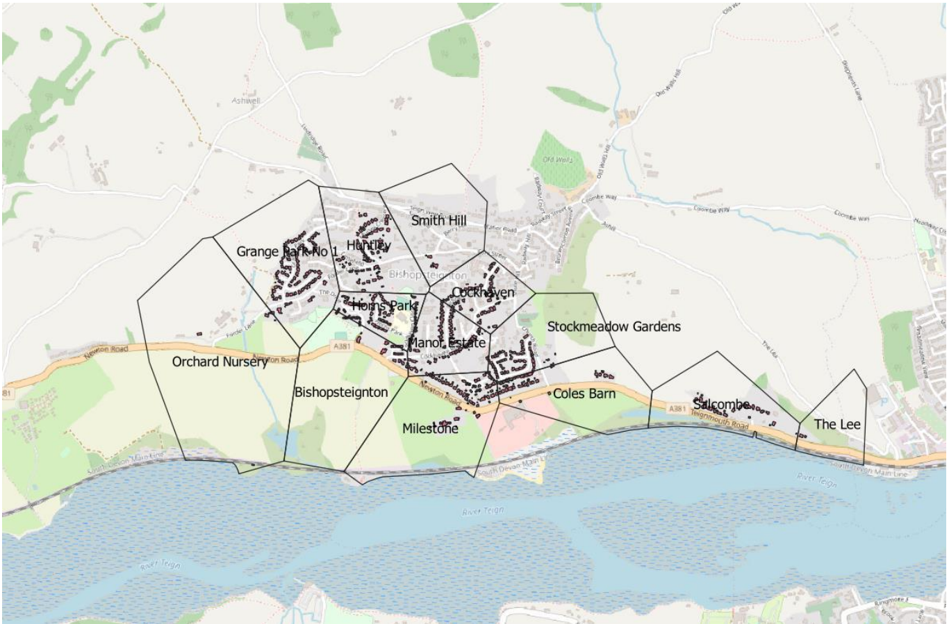
Figure 23: Map showing the shortlisted properties under consideration in Bishopsteignton and the secondary substations that supply these areas. Base map from ©OpenStreetMap contributors and Supply areas provided by National Grid Electricity Distribution, dataset
