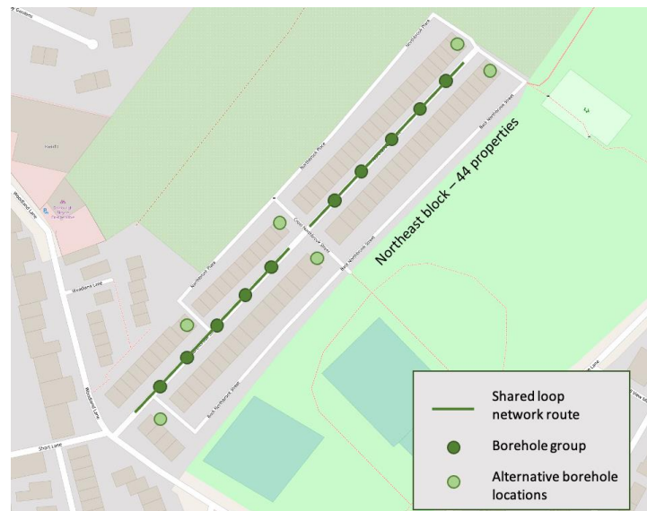
Figure 19 – Northbrook Street shared loop design used in detailed simulation studies.
