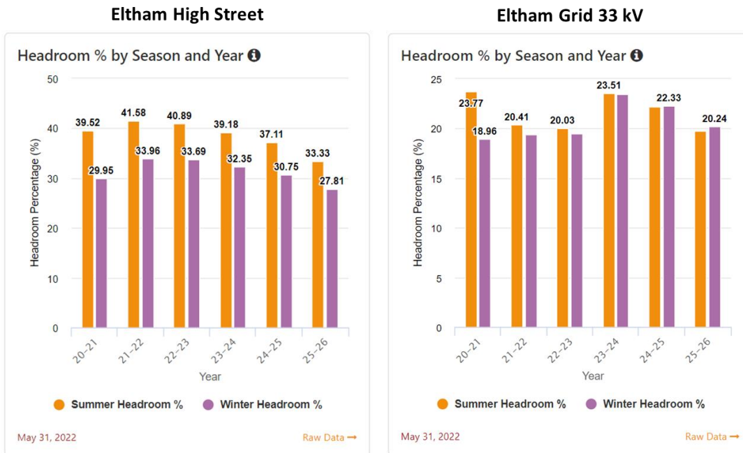
Figure 5.16. Primary substation capacities. Headroom data for the Eltham High Street and Eltham Grid 33kV primary substations that cover the areas of Greenwich being targeted. 36
