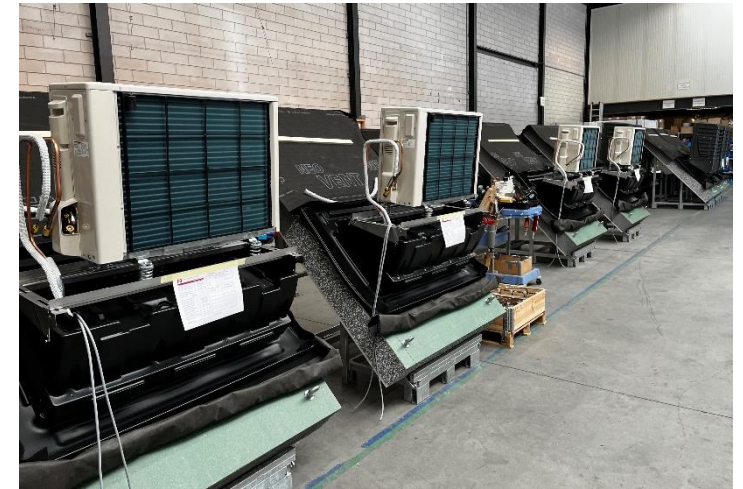
'Factory Zero' in Netherlands, a production line for roof-mounted air source heat pumps
